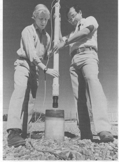
LOWERING an electronic borehole compass into a borehole are Bob Wayland (9114, left) and David Lee (7323). The new Sandia-developed tunnel detection techniques can help locate covert tunnels and abandoned mine shafts.
